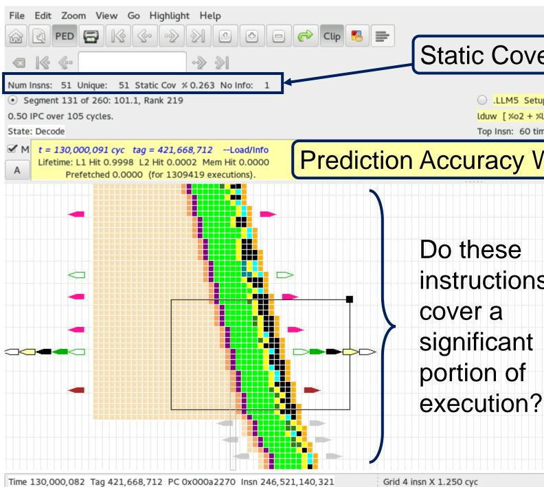
A pipeline execution diagram (PED) plot displa for each instruction, with the vertical axis I horizontal axis measuring clock cycles in the found to be incorrect from the result of branch for the correct branch and incorrect ones are d
